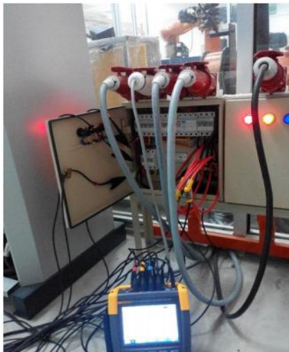
Figure 5: Fluke 435 Connected to KUKA KR 16 control unit
