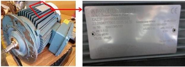
Figure 3.1: SEW Euro Drive Motor with Name Plate Source: Author
