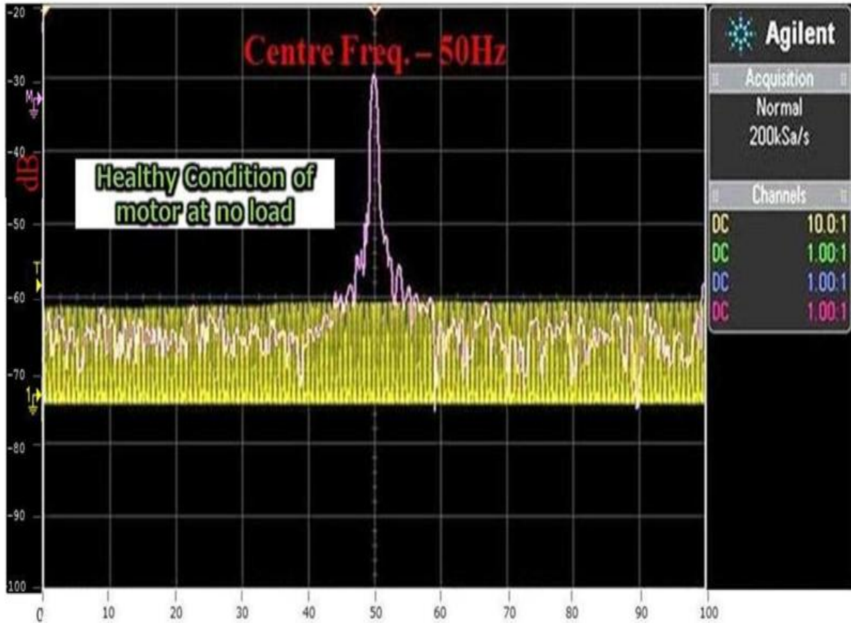
Figure 3.4: Spectrum for a SEW- EuroDrive Motor in healthy condition with no load
