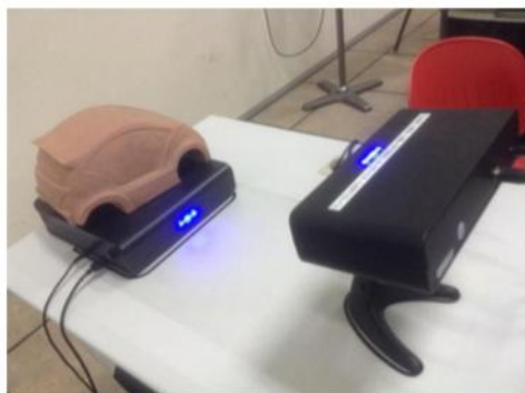
Figure 1 : Clay model of the concept design is scan using photogrammetry method.
