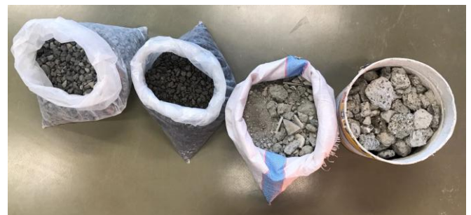
Fig 3: natural aggregate, recycled aggregate from batching plant, 8 year old aggregate and 16 year old aggregate (left to right)
