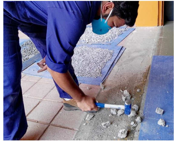
Fig 6: Hammering big pieces of aggregate to smaller pieces
