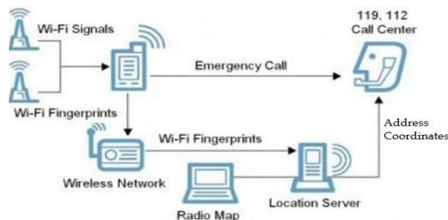
Fig. 1. Indoor Positioning System
