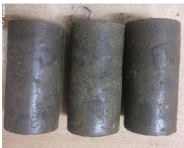
Fig. 7: Failure of 28 days cured sample of an optimum mix Variation in unconfined compressive strength for different GGBS content with a varying percent of bagasse ash is shown in fig. 8. Test resultsshow that 7.5 percent GGBS with 10 % BA mixed in a CH soil gives maximum strength.
