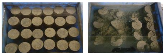
Fig.14: First wetting cycle of untreated soil
