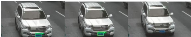
Fig. 6. Plate Detection (from left to right: one bounding box detected-true positive, two bounding boxes detected-false positive, no bounding box detected-false negative).
