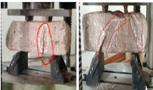
(a.) Without Reinforcement (b.) With Reinforcement Fig. 7 Testing of Model Beam – B
