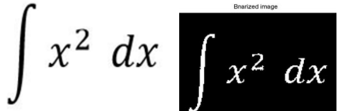
Figure 1. Sample Equation and its binarized representation
