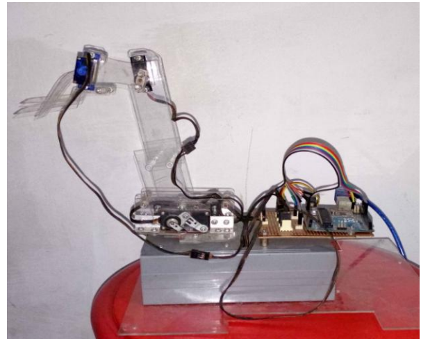
Fig. 2 Hardware of Robot Arm 4 DOF
