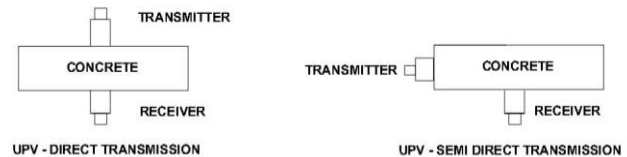
Fig.1 Propagating and receiving ultrasonic pulses
