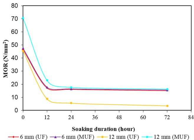
Fig. 4: Effect of soaking duration on the MOR of MDF bonded with UF and MUF resin.
