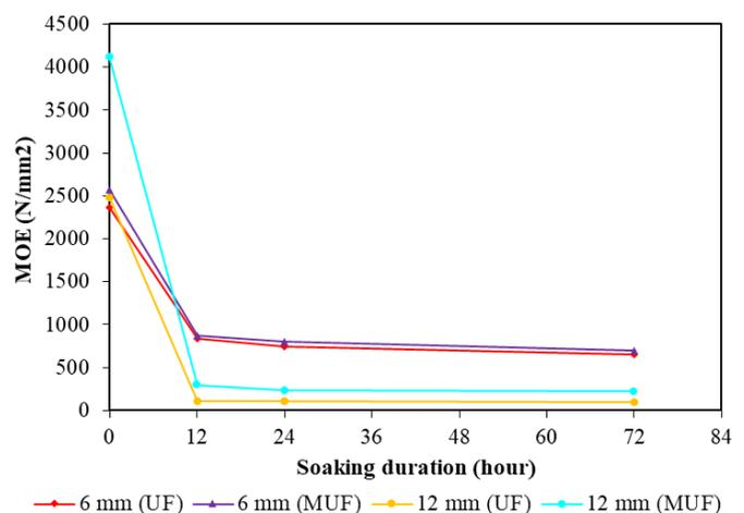
Fig. 3: Effect of soaking duration on the MOE of MDF bonded with different resin.
