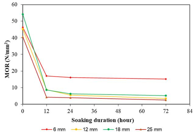
Fig. 2: Effect of soaking duration on the MOR of MDF at various board thickness
