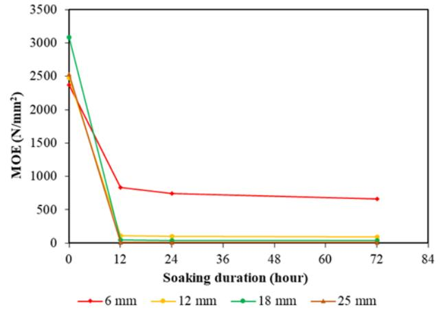
Fig. 1: Effect of soaking duration on the MOE of MDF at various board thickness
