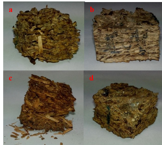
Fig. 2: Visual appearance of particleboards bonded with different binding agents after exposure to Coptotermus curvignathus : (a) 10% UF; (b) 10% UF + 20% PO; (c) 15% CA and (d) 15% CA + 20% PO + 20% FA
