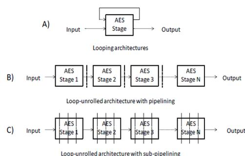
Figure.1. AES structural design
