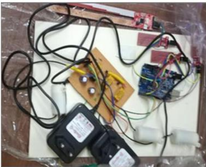
Figure 5. Node MCU connected to the sensors
