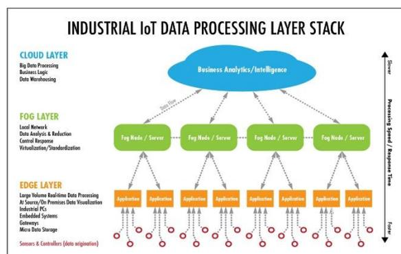
Fig 1 Layered architecture of Fog Computing
