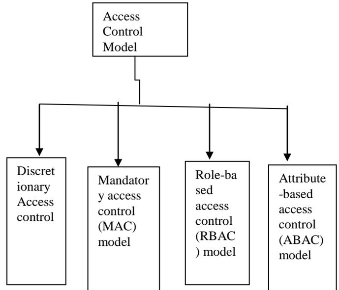
Fig 8: Types of Access control model
