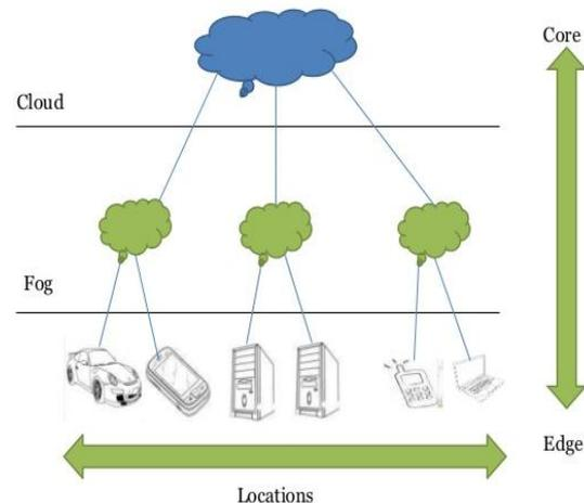
Fig 2. Relationship between cloud, Fog and Edge devices
