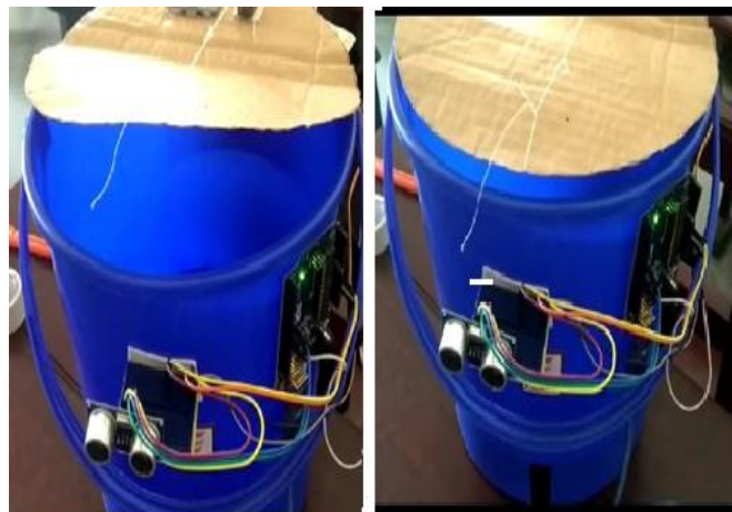
Figure 5: Smart bin with automatic lid open
