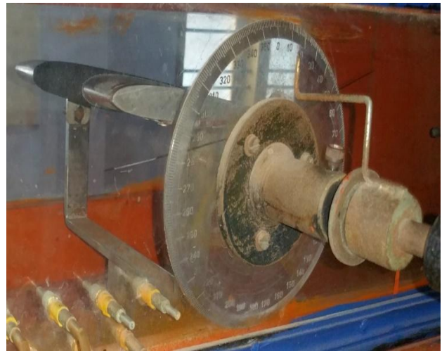
Fig. 9: Testing of wing with surface roughness
