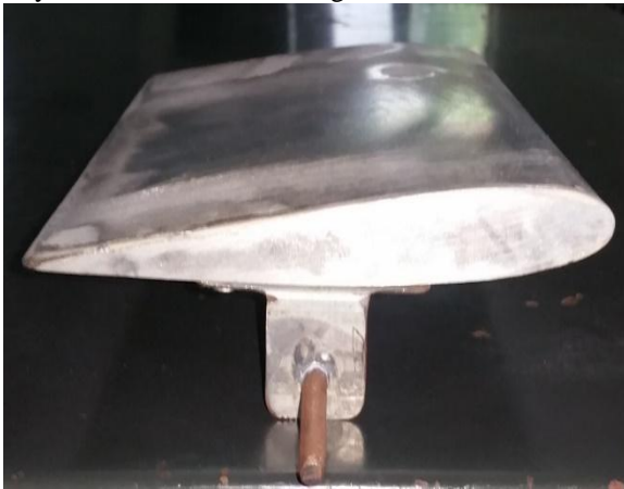
Fig. 4: Fabricated wing model without roughness
