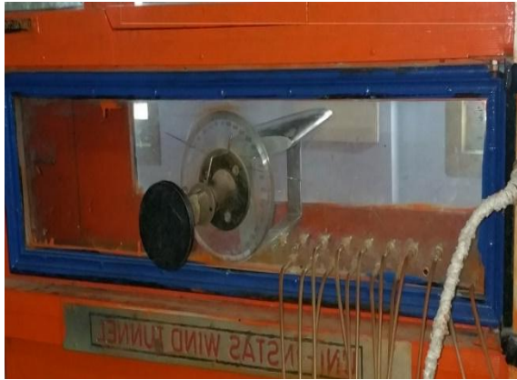
Fig. 7: Testing of wing without surface roughness
