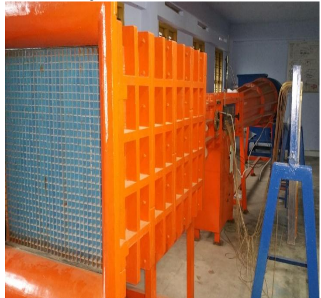
Fig. 6: Subsonic wind tunnel
