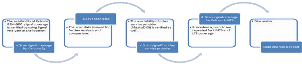
Figure 4: Signal strength measurement procedure
