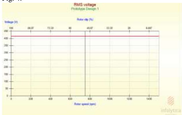
Fig. 4. Supply voltage vs Rotor speed for conventional motor.
