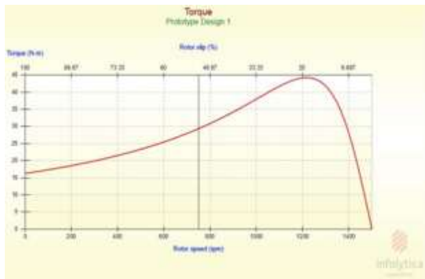
Fig. 10. Torque curve of altered motor.
