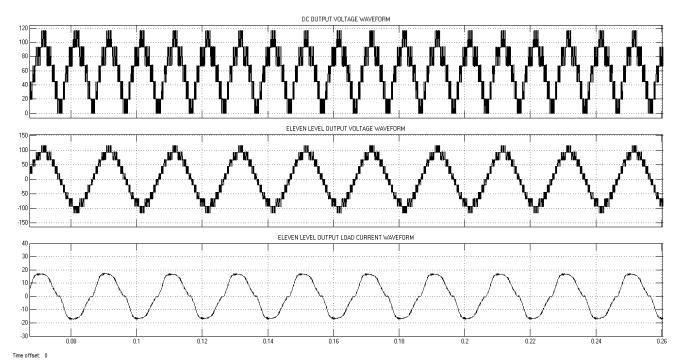
Fig.11. Eleven level output before filter, voltage vs time (matlab Simulink)
