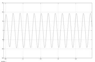
Fig.12.Eleven level output after filter, voltage vs time (matlab Simulink)
