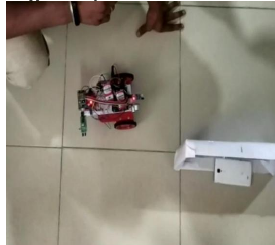
Figure 6: Car Detected a slot on its Left Side
