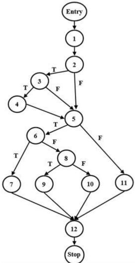
Fig. 1: CFG for Triangle Program Classifier
