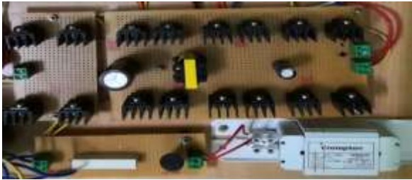
Fig.12 Solid state transformer
