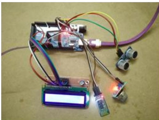
Fig 4. Gas detection system integrated with ultrasonic sensor and LCD panel.
