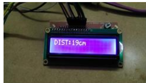
Fig 6. Distance calculated by ultrasonic sensor
