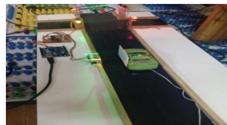
Fig. 6 Ambulance is sensed by RFID reader
