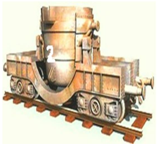
Fig. 1 Ladle Car ready for transportation
