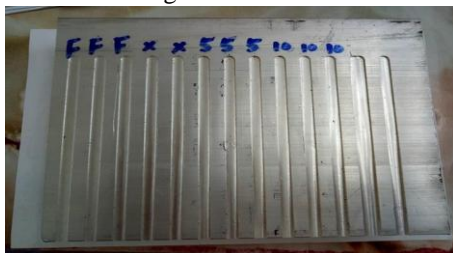
Fig. 6: Milling Process Is Undergone On The Aluminium Block
