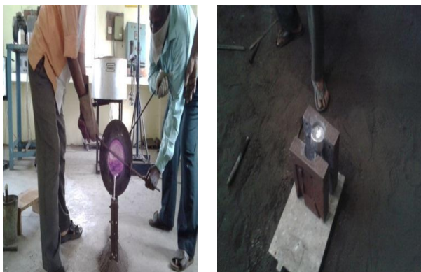
Fig.2 Casting Procedure for ZA43/B 4 C composites
