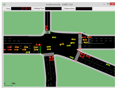
Fig. 6. SUMO graphical user interface demonstration with a running simulation of an intersection. Color of the cars represent their speed: red – complete stop, green – 54 km/h.
