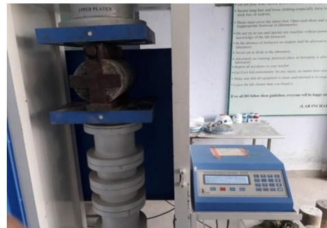
Figure 6: Split Tensile Strength test at Advanced Material Testing Lab, Integral University, Lucknow.
