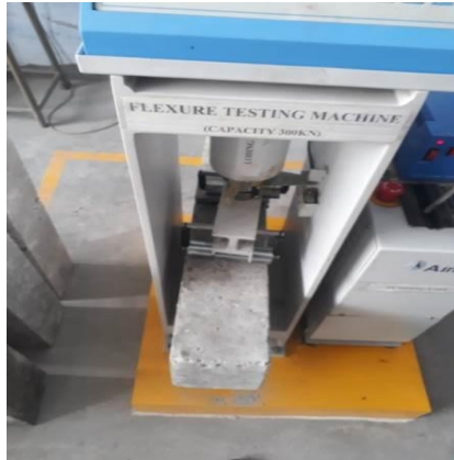
Fig. 9: Flexural Strength Test at Advanced Material Testing Lab, Integral University, Lucknow
