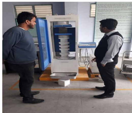
Fig. 3: Testing for Compressive Strength at Advanced Material Testing Lab, Integral University, Lucknow
