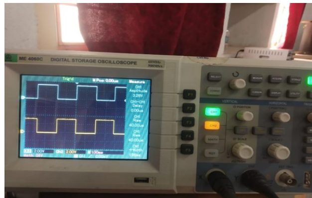
Fig.11 Pulses by using DSP technique
