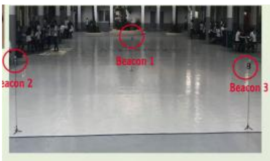
Fig. 5: Beacons are placed in a triangular manner
