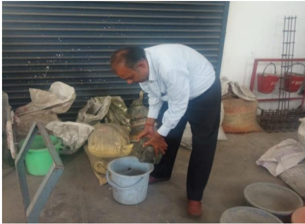
Fig.7: Saturated Water Absorption Test
