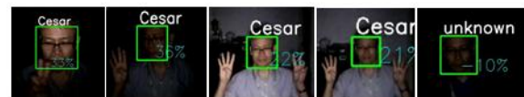
Figure 5: Sample images of detected faces at different distances and illumination successfully recognized by the face recognition algorithm. One image in the example is not recognized successfully.
