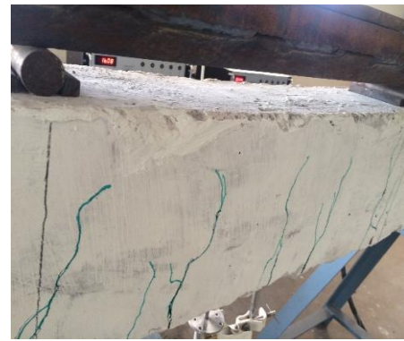
Fig 5: Failure Pattern of the beams
