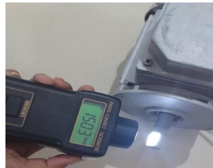
Figure 19. Three-phase Induction motor speed with VFD
