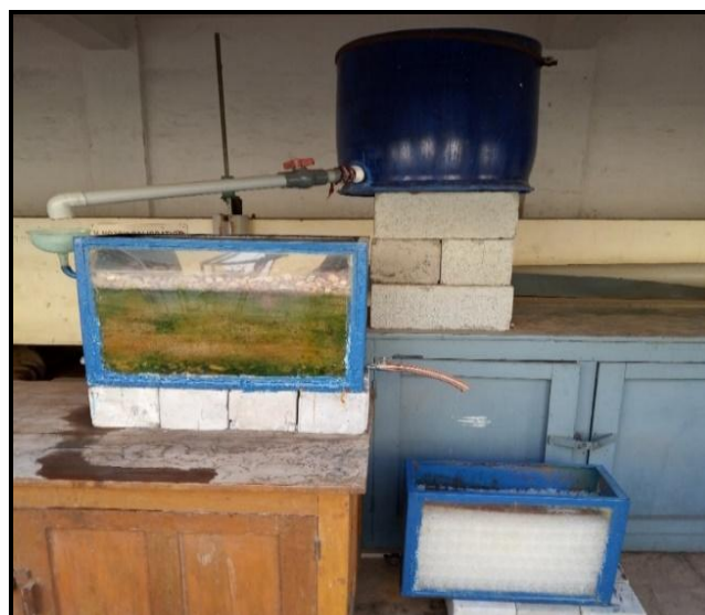
Fig 6. Working Model of Greywater Treatment System
