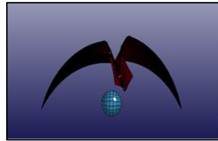
Fig.5: Deformation of the semi-circular, 2 Layers, [0/90] specimen
