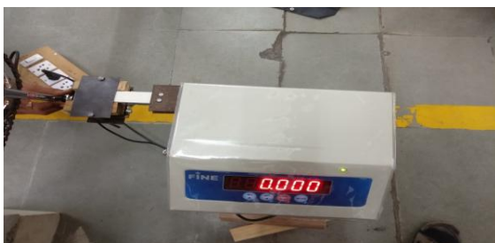
Fig. 3: Load Cell with fixture and Indicator
