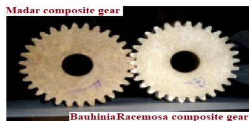
Fig.6. Madar And Bauhinia Racemosa Composite Gears
