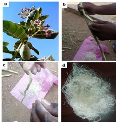
Fig.1. (a- d) Extraction process of Madar fibers
