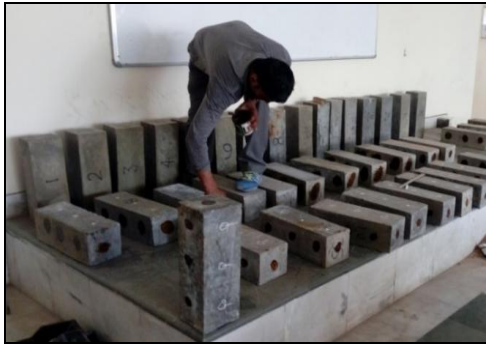
Fig. 2 Applying grease to ensure adequate acoustical coupling between concrete surface and face of the transducer at points of test
