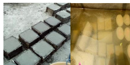
Fig 5: prisms setting and curing
