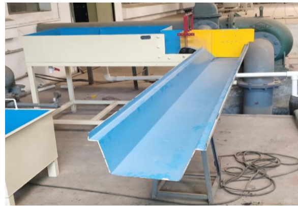
Fig.3: Photograph of Side channel spillway model.
