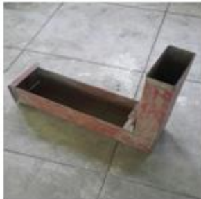
Figure3 L-Box Test Setup
