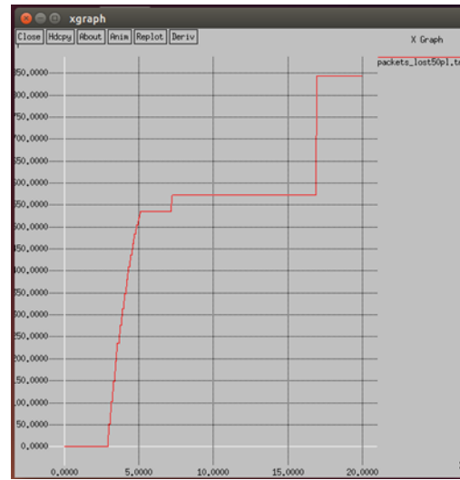
Fig 5 shows packet lost for 50 nodes of the Enhance AODV
