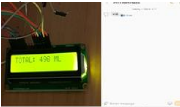
Fig 4(b): Display of amount of fuel poured in to the tank
