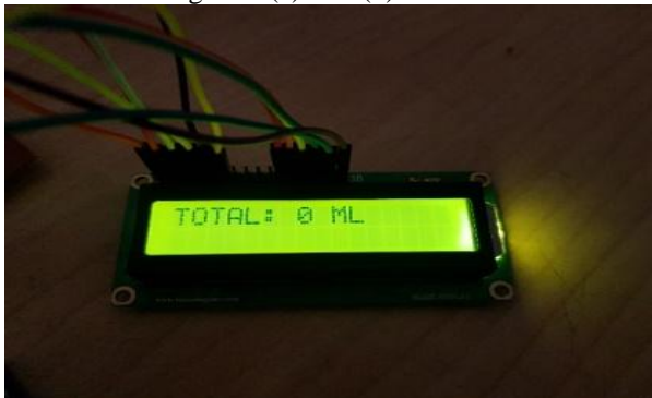
Fig 4(a): Display of no fuel is filled in the tank
