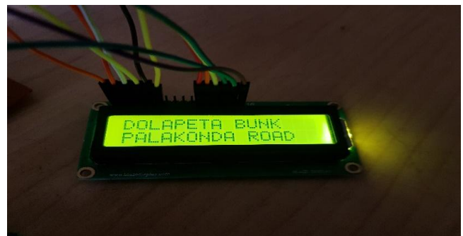
Fig 4(d): Display of nearby fuel station
