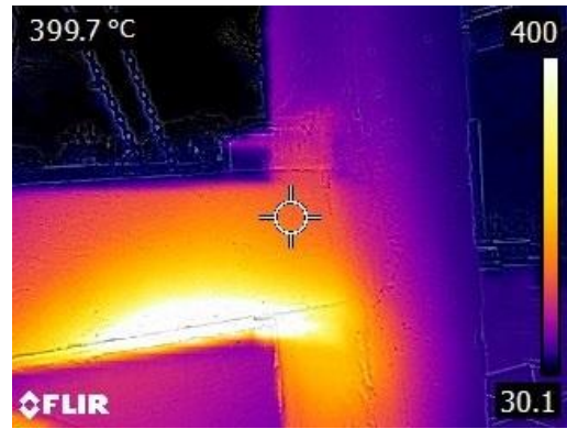
Figure VII - Temperature variation near Hybrid Connection
