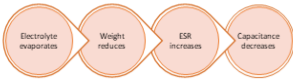
Figure 3: Failure criterion of electrolytic capacitor
