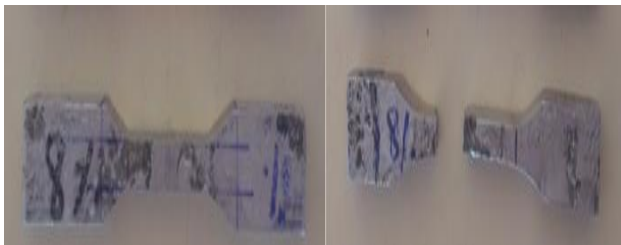
Figure 5. Before and after fractured tensile test specimen
